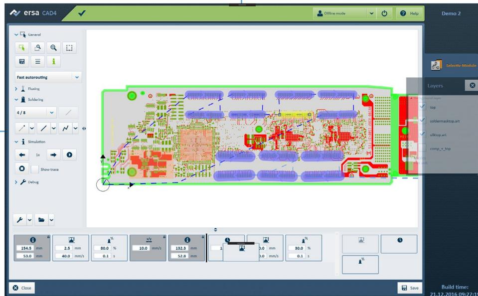
(axis 1 or 2) to the soldering spots. The optimum workflow for fluxing and soldering is automatically calculated by an autorouting function. Alternatively, the operator can define the soldering point sequence manually.
