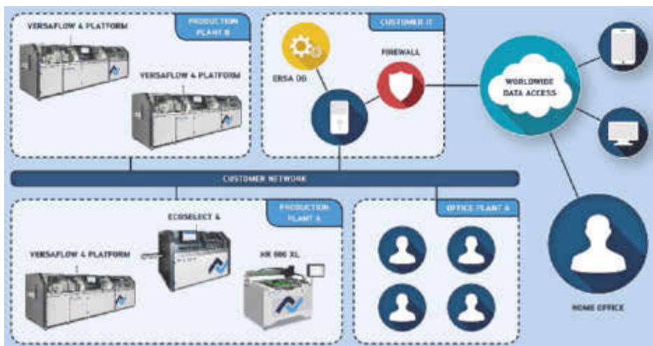
Structure for integrating soldering systems in the company IT.
